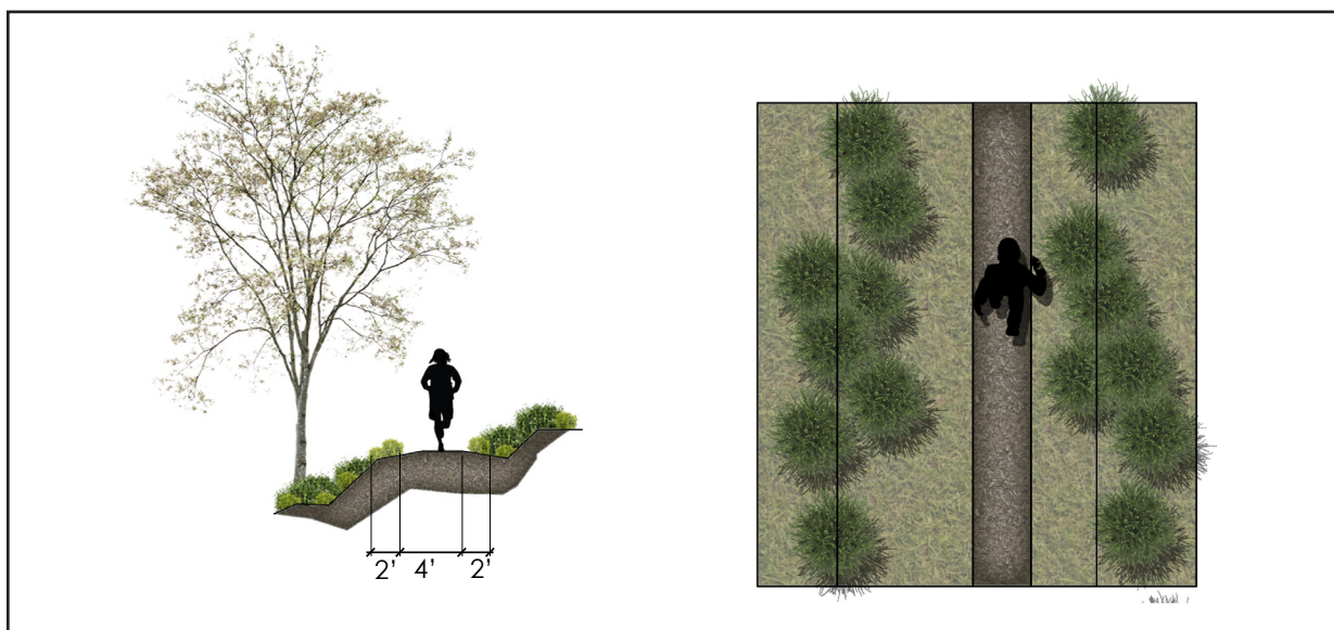
Figure 44: Typical cross section (left) and plan view (right) of a backcountry trail.
